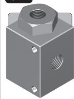
The SV25 is a 1/4" ported shuttle valve. The valve will sense the higher of two pressures and send this pressure to the outlet. The valve is often used to provide redundancy on pilot systems. In the event of pressure loss on one inlet, the valve will automatically switch to the higher pressure supply.
