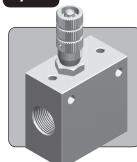
The MF75 is a 3/4" nominal bore flow metering valve, adjustable via a micrometer style handle. The valve is marked with a preferred direction of flow, but it may be used in the opposite direction to provide bi-directional speed control of a cylinder or actuator, although the level of metering will vary depending on direction.
