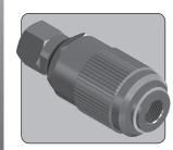
The IMC50 is a 1/2" nominal bore metering valve with a reverse free-flow check function. It provides metered flow in one direction, and free flow in the opposite direction. It is ideal for uni-directional speed control of a cylinder or actuator. The valve may also be referred to as a flow control
