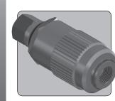
The IMC37 is a 3/8" nominal bore metering valve with a reverse free-flow check function. It provides metered flow in one direction, and free flow in the opposite direction. It is ideal for uni-directional speed control of a cylinder or actuator. The valve may also be referred to as a flow control
