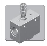
The CMF100 is a 1" nominal bore metering valve with a reverse free-flow check function. It provides metered flow in one direction, and free flow in the opposite direction, ideal for uni-directional speed control of a cylinder or actuator.
